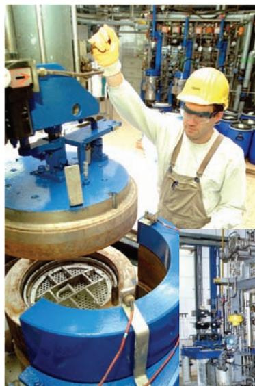
*The SFE process consists of exposing starting material and carbon dioxide to very precise pressure and temperature settings; the botanical raw material is first loaded in a vessel (pictured in two views), while temperature and pressure is increased, allowing the  $\text{CO}_2$  to reach supercritical stage; photos courtesy of Evonik.*
