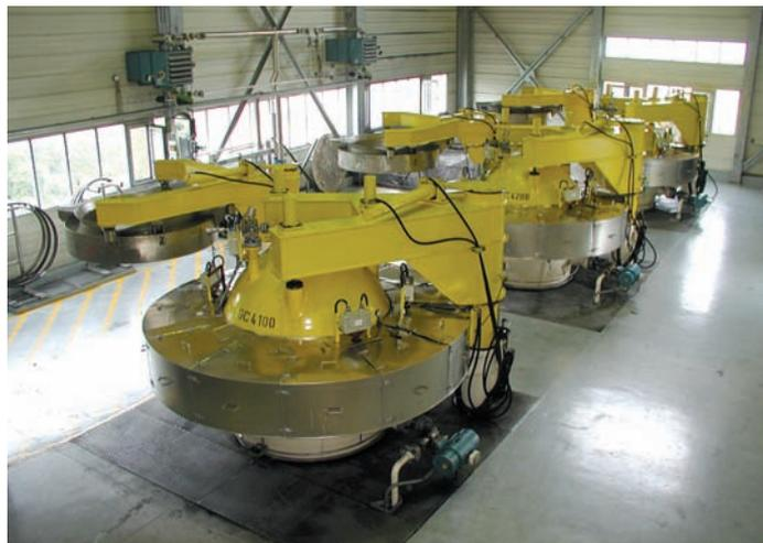
*Beginning in the 1980s, large-scale high-pressure SFE units—three of which are shown here—were aimed at the decaffeination market; in parallel, other applications were found, including the extraction of hops flavor and bitter compounds for the beer industry; photo courtesy of Evonik.*
